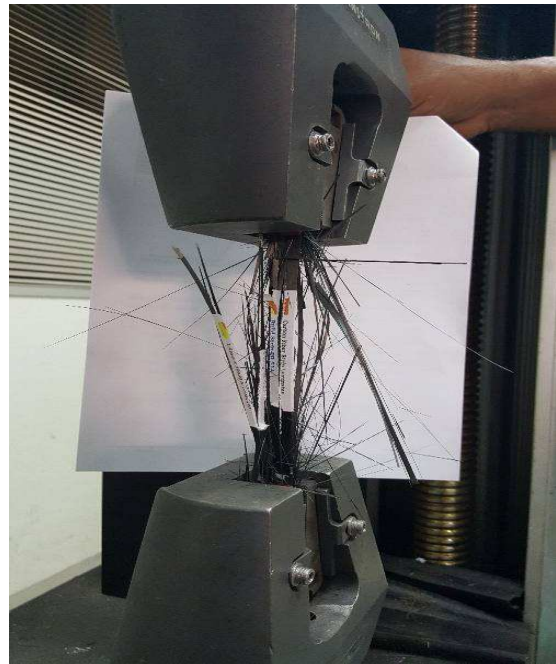
Testing Equipment, Method of Tester Installed, Once Tested the CFRP Cured Laminates Breaking
