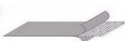
PVC P polyester fiber mesh reinforced
